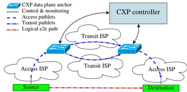
Figure 1: The CXP stitches QoS-enabled e2e paths.
